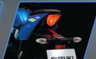
Tail Light and LED License Plate Light
